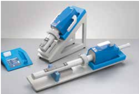
Measurement in bores
