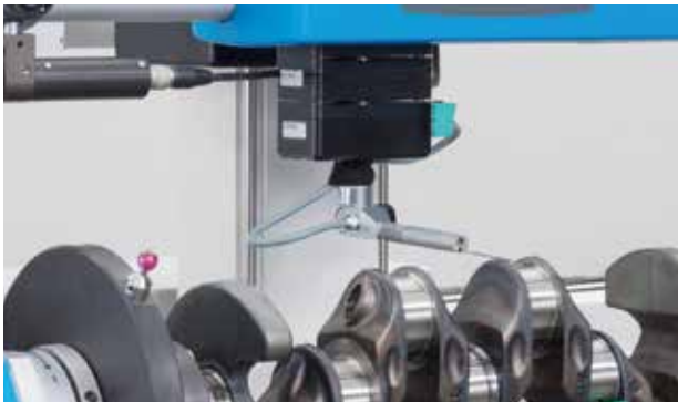
The probe is swiveled by 90° for roughness measurements on pin bearings
